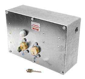
The Type TDKRU is designed to permit removal of the initially held (or secondary) interlock key after insertion of a primary key and the elapse of a predetermined time delay. The TDKRU is comprised of two key interlocks, a timing device, a solenoid, and a signal light for indication.
